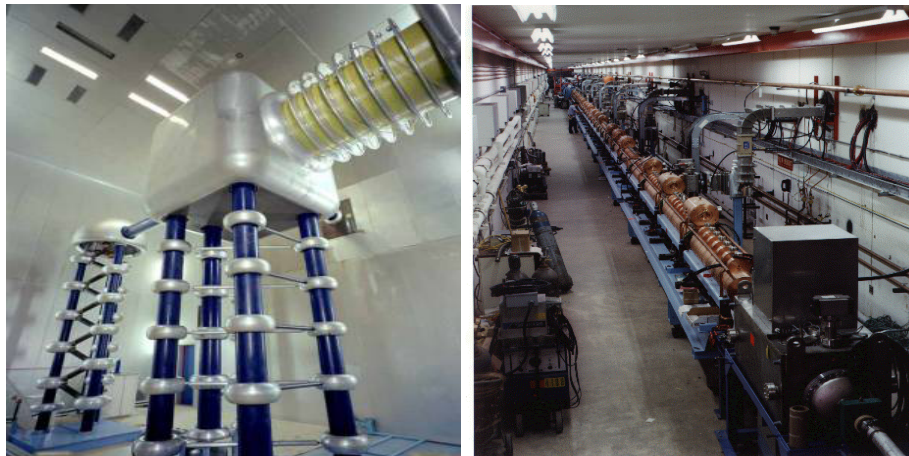
Figure 2.2: The Fermilab's Cockcroft-Walton preaccelerator and Linac
